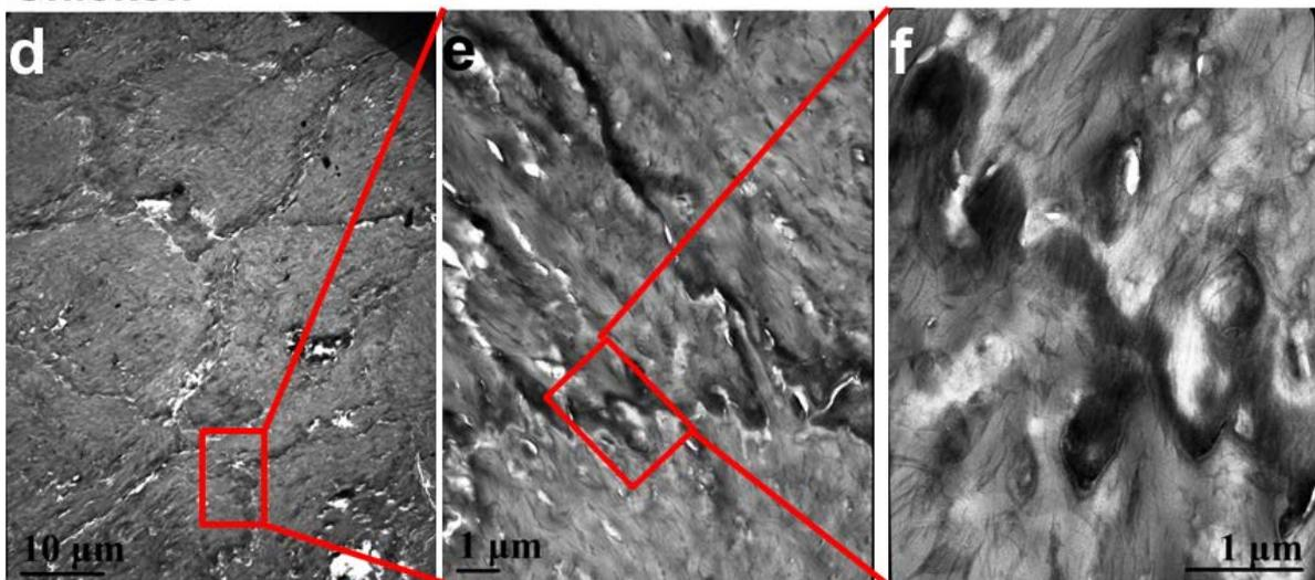
**Figure 5.** Transmission Electron Microscope images of the woodpecker's and chicken's rhamphotheca from the very tip of the beaks in a cross-sectional view: (a) keratin cells of the woodpecker; (b) regular wavy lines of the keratin cell boundary; (c) wavy boundary and fibers; (d) keratin cells of the chicken beak; (e) irregular wavy lines of the keratin cell boundary; (f) boundary and fibers.
