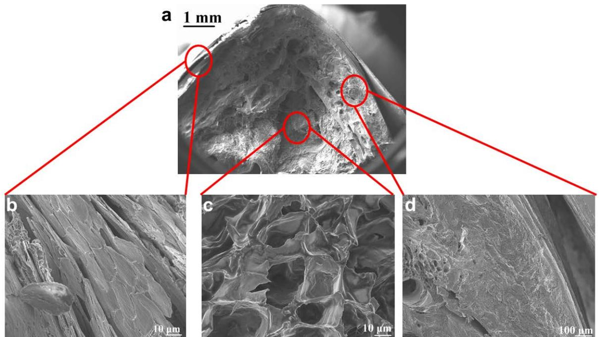
**Figure 4.** Microstructure of the upper beak of the chicken garnered from Scanning Electron Microscopy shows (a) a cross-section view of the entire fractured area, (b) an exterior rhamphotheca layer comprised of  $\beta$ -keratin scales, (c) an inner foam, and (d) an interior bony layer.
